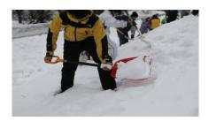
By gripping Dig-Log when shoveling snow, users can find out the weight of the snow they move and the calories they've burned.
